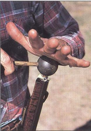
Center the round ball on a pre-lubed patch on the barrel. Use the short end of the ball starter to push the ball flush with the muzzle. Then push ball several inches further down the barrel with the longer rod, and finally, seat the ball on powder with the ram rod.
